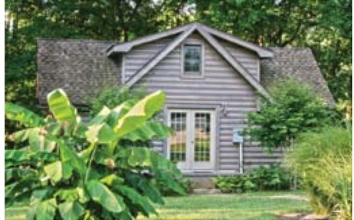
The cabin was built from a custom design, using Honest Abe's 8" x 8" D-Log profile, offering exceptional energy efficiency. It also features the company's Heavy Timber Roof and Ceiling Systems, which utilized large exposed beams for its structure. The family chose to use Lifeline Ultra-2 in Driftwood by Perma-Chink Systems for the stain, providing a washed and naturally weathered look to blend into the farm and river surroundings.
