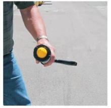
Attach the end cap and cone tip to the end of the barrel. Make sure the tip of the cone is cut to the diameter of the bead you want to apply.
