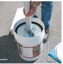
Place the follow plate on top of the Remove the cap and cone tip from the barrel onto the lip surrounding the hole in the middle of the Follow Plate. Make sure the gun is perpendicular to the plate, and there is a tight seal between the barrel and the O-ring. If the barrel is tilted air will be sucked into the gun during the loading process.
