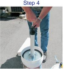
Depress the rod release plate and Once the rod is fully extended and draw back the rod with a smooth, the barrel is full of product, give the even pull. Make sure the barrel trigger stays flush with the plate and don't disengage the barrel from the tilt the gun as you pull the rod back. Follow Plate with a twisting motion.
