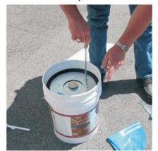
To remove the Follow Plate from an empty or partially full container, insert the handle rod into the open nut on the surface of the plate and pull it out.
