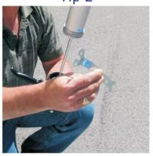
If the gun begins to suck air, tighten the blue base with the wrench that comes with the gun.
