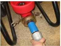
Slide out the stator tube & pump housing retainer assembly.
