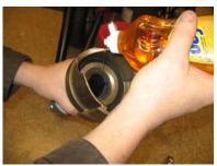
Thoroughly lubricate the inside of the stator tube with liquid dish soap.
