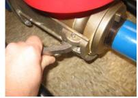
Release locking cam ears on the pump housing base.
