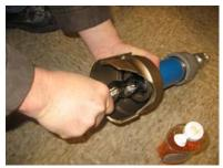
Screw and push the rotor into the stator tube, counter-clockwise.
