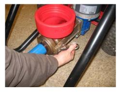
If the rotor is inserted far enough and the connecting drive shaft is aligned, the assembly will connect back into it's original position and can be locked back in place. The Rotor-Stator Assembly is complete.
