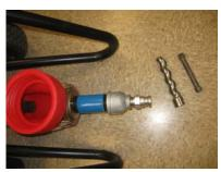
Unwrap rotor and connecting driveshaft.
