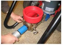
Slide the rotor-stator assembly into the pump housing base. If the assembly does not go all the way back, check the connecting drive shaft alignment.
