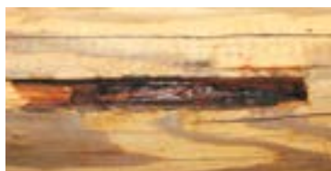
Wood fibers consolidated with M-Balm
