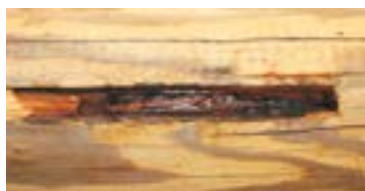
Wood fibers consolidated with M-Balm
