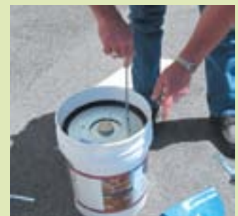
Insert the handle rod into the open nut to remove the follow plate
