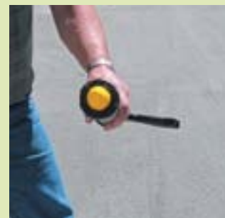
Attach the end cap and cone tip to the end of the barrel
