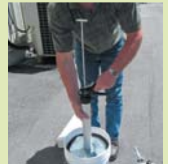
Ensure the tight seal, fully extend rod and fill the barrel. Disengage from the follow plate
