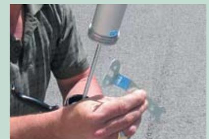
If the gun begins to suck air, tighten the blue base with the wrench that comes with the gun.
