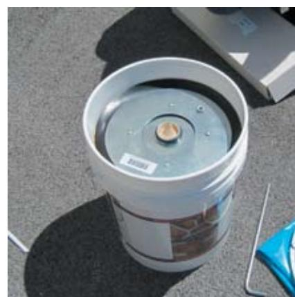
Place the follow plate on top of the chinking in the pail making sure that there is a good seal between the wall of the pail and the flexible edges of the follow plate.
