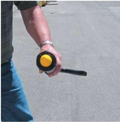
Attach the end cap and cone tip to the end of the barrel. Make sure the tip of the cone is cut to the diameter of the bead you want to apply.
