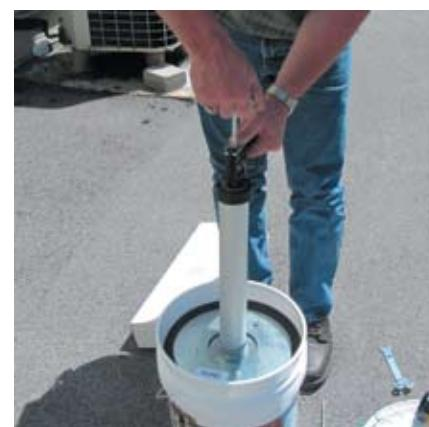
Depress the rod release lever and draw back the rod with a smooth, even pull. Make sure the barrel stays flush with the plate and don't tilt the gun as you pull the rod back.
