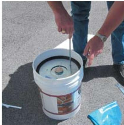
To remove the follow plate from an empty or partially full container, insert the handle rod into the open nut on the surface of the plate and pull it out.
