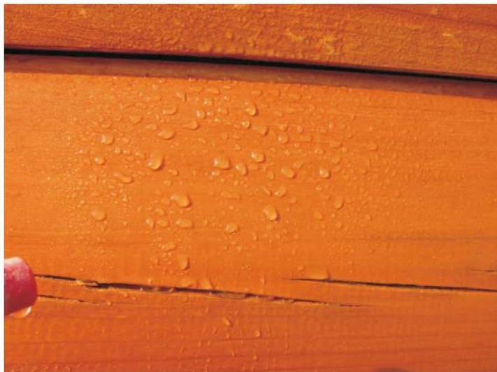
Water beading on a finish that contains wax.
