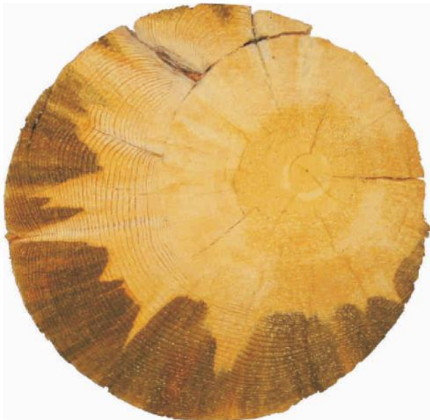
Cross section of blue stained log
