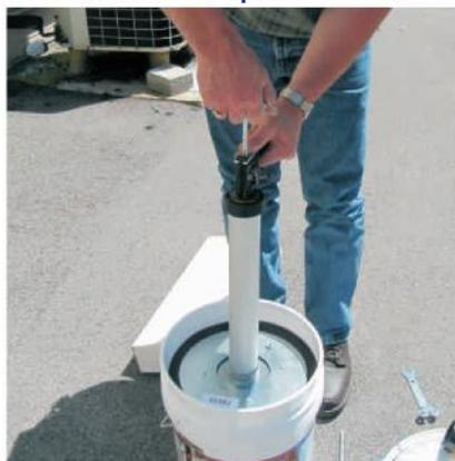
Depress the rod release plate and draw back the rod with a smooth, even pull. Make sure the barrel stays flush with the plate and don't tilt the gun as you pull the rod back.
