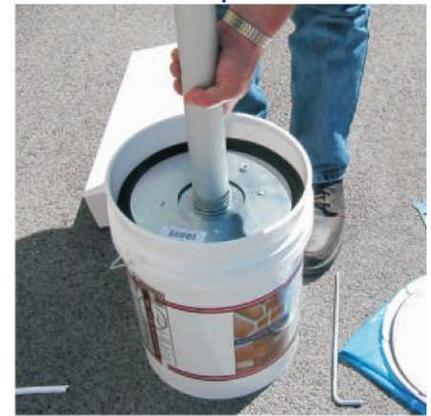
Remove the cap and cone tip from the end of the Cox gun barrel and ensure that the rod and plunger are fully forward. Push the end of the barrel onto the lip surrounding the hole in the middle of the Follow Plate. Make sure the gun is perpendicular to the plate, and there is a tight seal between the barrel and the O-ring. If the barrel is tilted air will be sucked into the gun during the loading process.
