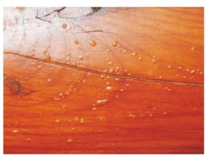
The wood may look clean and bare, but in reality the old oil carriers may still be in the top layer of wood. With the application of the first coat of LIFELINE<sup>TM</sup> these oils are now trapped in the wood. Yes, water vapor can permeate our finishes. However, oil molecules are much larger and can not pass through, reducing the films ability to transmit water vapor in and out of the wood.
