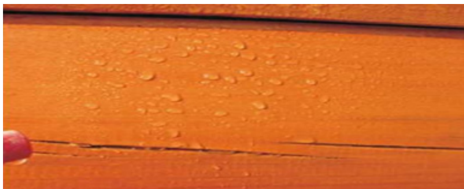
Water beading on a finish that contains wax
