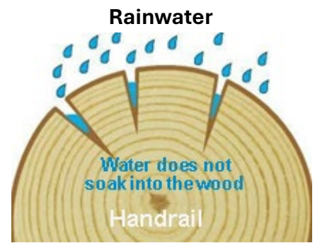
Finish film on wood surface and in fissures.
