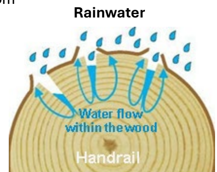
Finish film on wood surface but not in fissure.
